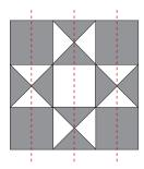
**4.** The Brick border can be moved in all directions by 2" (50,8mm) to the next half tile i.e. square or triangle, to accommodate irregular shaped rooms, as long as the overall look is balanced.
